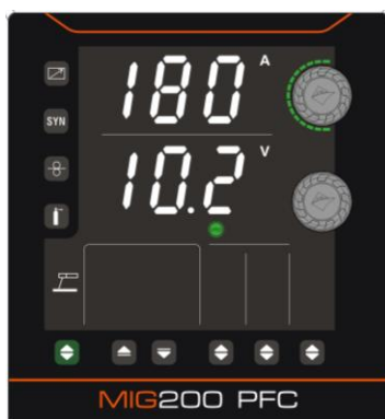
(Select MMA mode in HD digital screen)
